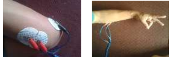
Fig -3 (a): Electrode placement (b): User performing gesture during the testing
