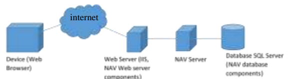
Fig 2: Web Client Network Architecture (K. Dhinsdsa et. al, 2013)
