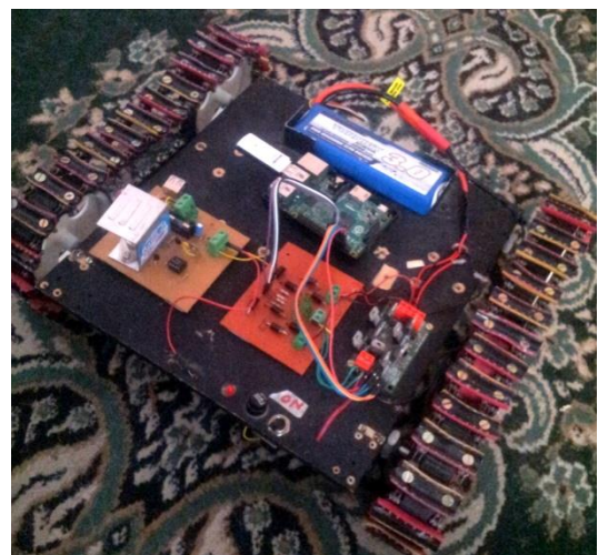
Fig 5.1. The tread-bot designed for taking images by clamping a smart phone to the chassis
