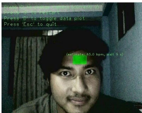
Figure 4: Determining the area of pixel to analysis the BPM
